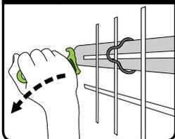
Withdraw the Driver leaving the KwikAz clip attached to the containment screening and the pole/standard.
