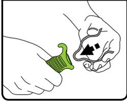
Insert the KwikAz clip into the jaws on the front of the Driver and push down until fully engaged.
