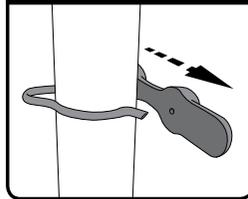
Slide the hole of the cap over the first exposed point of the clip and push down. Stretch the tab across.
