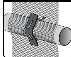
Strike the clip through the netting/shade cloth onto the scaffolding/fencing as per normal operation.
